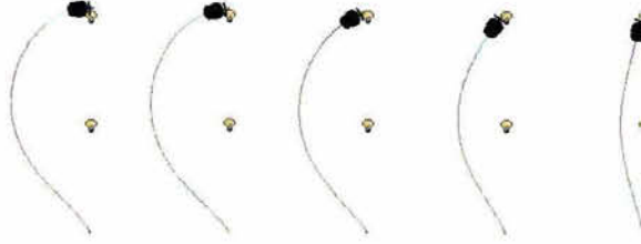
Figure 3. Trajectories of the robot with different energetic cost per step, from left to right: 20, 100, 200, 300, and 400.
